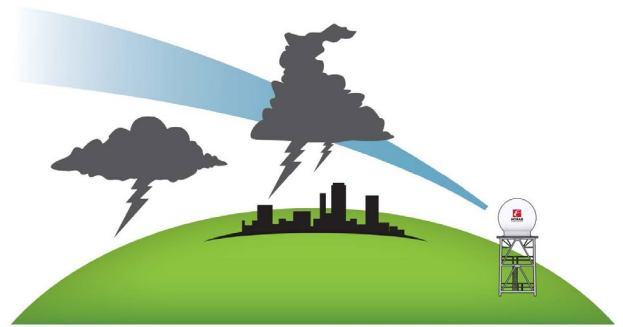
Figure 7 - Proper positioning of the radar means that the focus of the signal is over the observed area.
