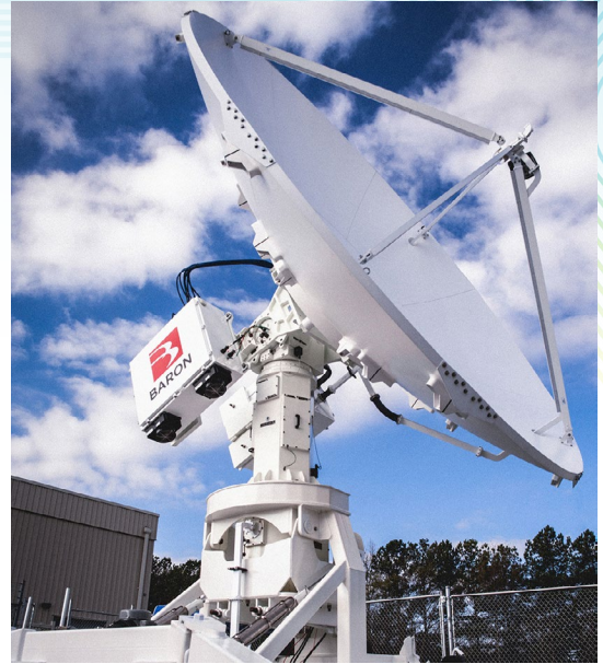
Figure 8 - Baron delivered this C-band dual-polarization radar to the U.S. Department of Energy.
